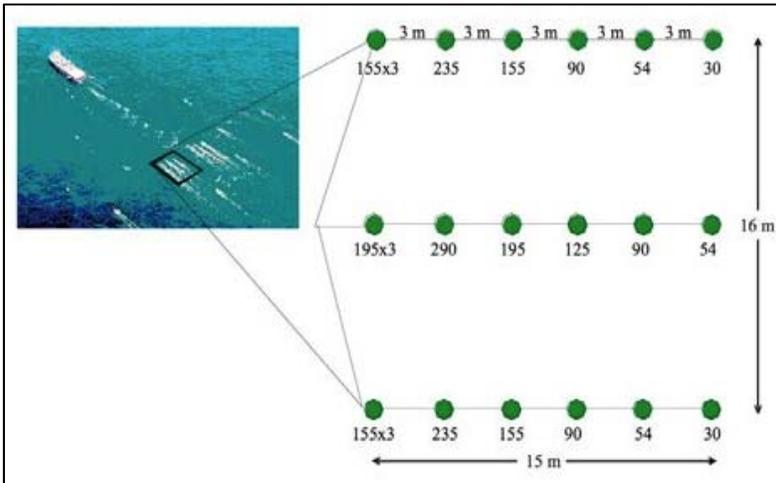
Figure 1. A typical seismic array geometry, illustrating the spacing between elements. As in this figure there are usually two such arrays towed side by side and triggered in alternation while the other array is re-pressurizing.
