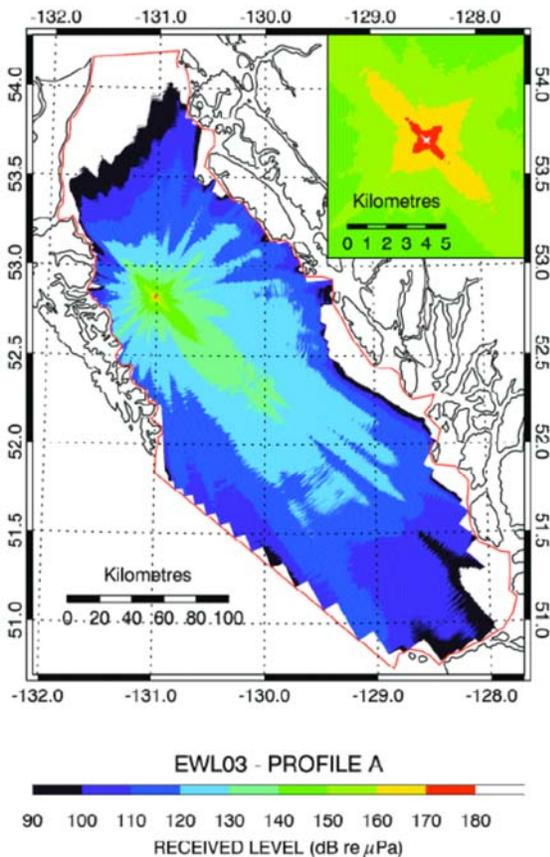
Figure 6. Modeled propagation loss for a seismic array operating in the Queen Charlotte Basin, British Columbia (from MacGillivray, 2007).
