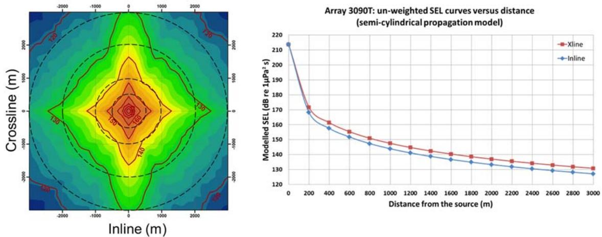
Figure 5. Modeled lateral transmission loss from a typical seismic array (Source: Goertz et al 2013, EAGE First Break).
