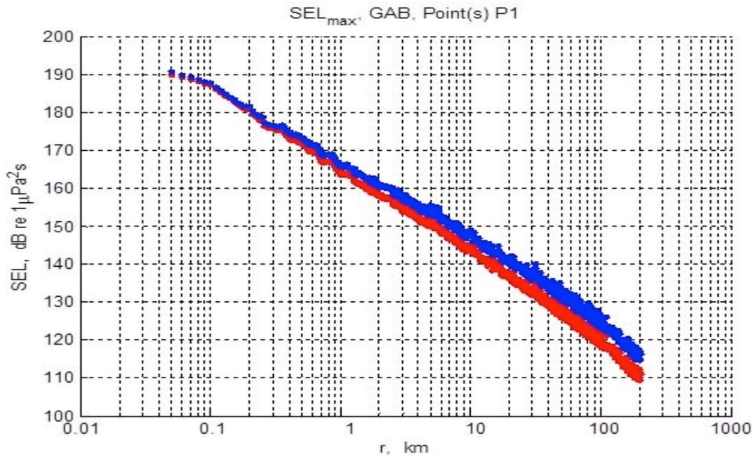
Figure 7. Modeled sound attenuation plots of 4130 in<sup>3</sup> (blue) and 3090 seismic arrays generated for a constant water depth of 100m in the Great Australian Bight (Source: R. McCauley, Curtin University).
