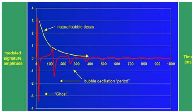
Figure 2. A plot of pressure or amplitude (vertical axis) versus time (horizontal axis) of a single source, referred to as an air-gun’s pressure signature. It shows the first, or primary, positive pressure pulse due to the initial expansion of the bubble that is created by release of compressed air. The subsequent lower amplitude pulses in red are known as the “bubble train”.
