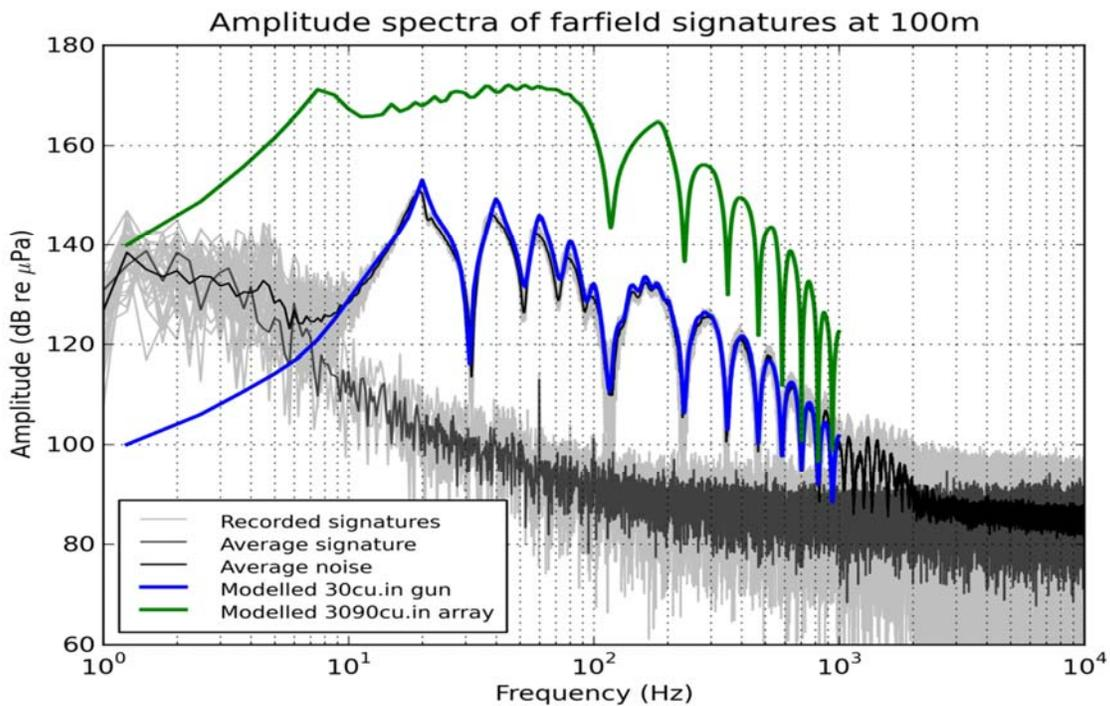
Figure 8. Modeled and measured frequency-specific amplitude for a 3090 cubic inch array (modelled) and a 30 cubic inch single source (modeled and measured). The measurements were made in a quiet fjord environment in Norway by a
