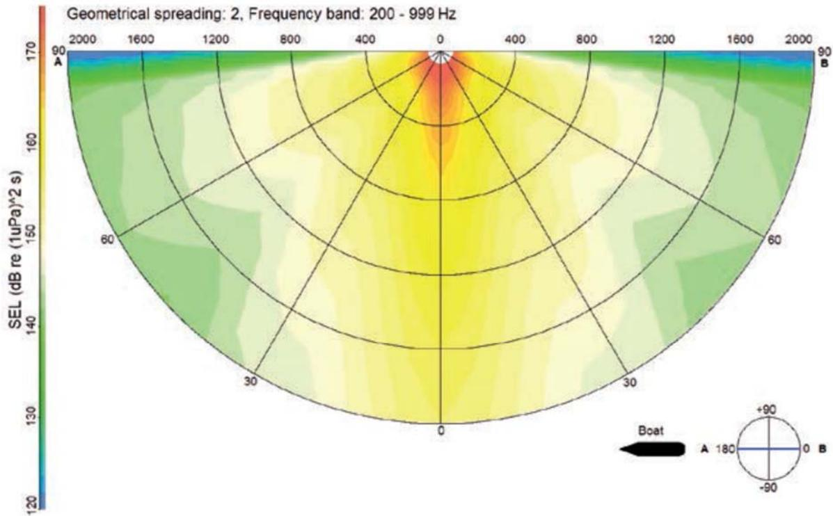
Figure 4. Polar plot of modeled 3080-in<sup>3</sup> source, looking downward and in cross section from port (-90) to starboard (+90), illustrating the directionality of the array output; with highest sound levels in red (170 dB) and lowest in blue (120 dB). Numbers across the top are distance from the sound source in meters. (Source: Goertz 2013).
